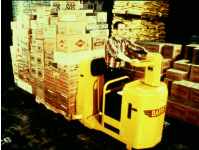
Figure 21.16. Example of Order Picking in the Aisle to a Vehicle with Double Pallet Trailer
