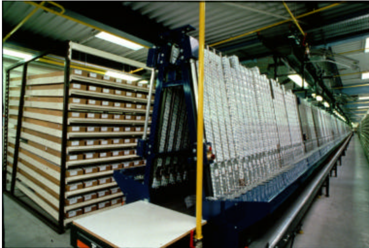
Figure 21.2. Automatic Order Picking A-Frame (Picture courtesy of Electrocom)
