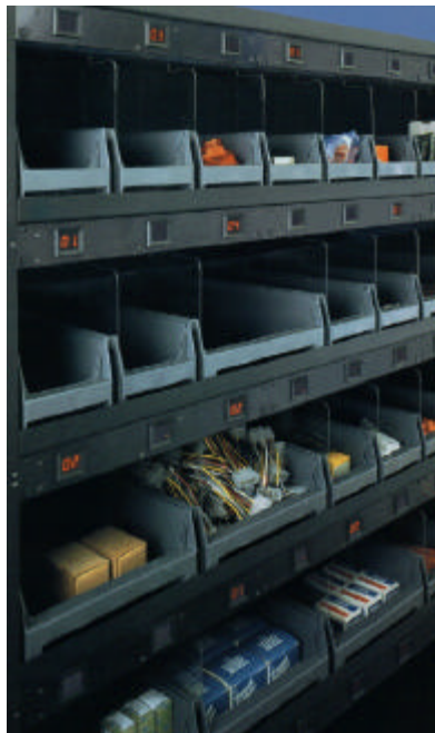
Figure 21.7. Quantity LED Displays on Shelves (Pick-To-Light) (Photo Courtesy of AutoPick)
